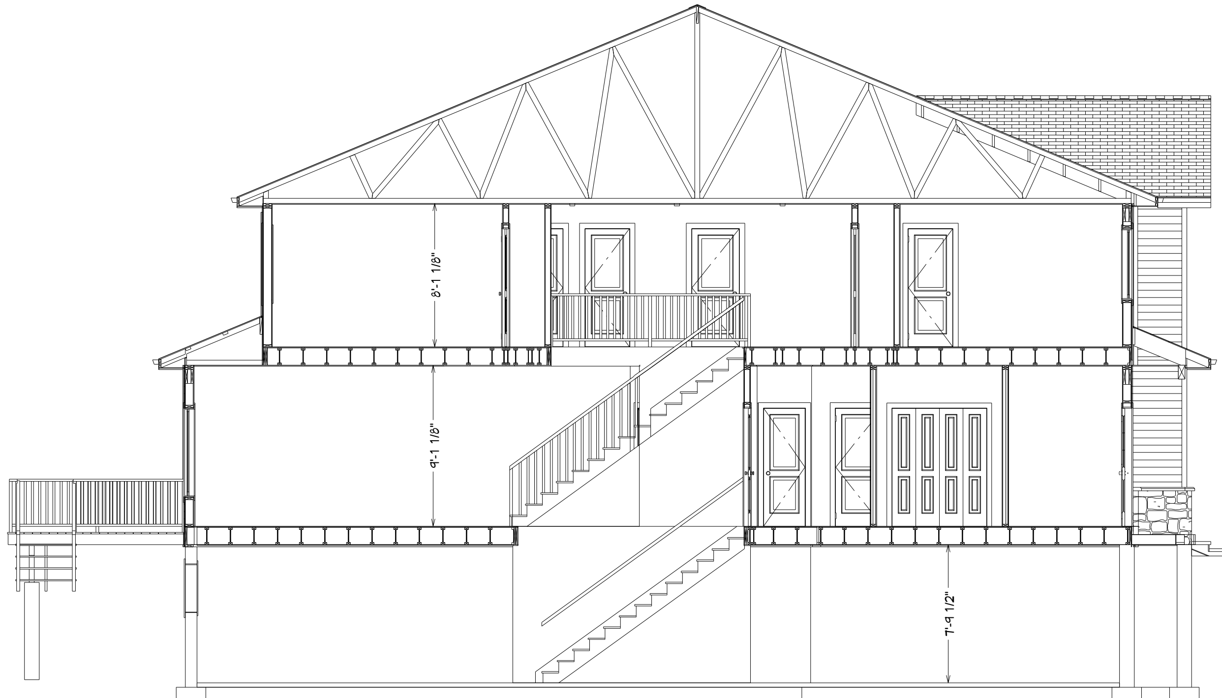
(E5) Cross Section - Stairwell
