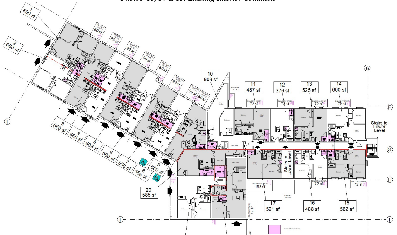
Figure 5: Schematic Main Level Floor Plan of Proposed New 34 Unit Adaptive Re-Use
