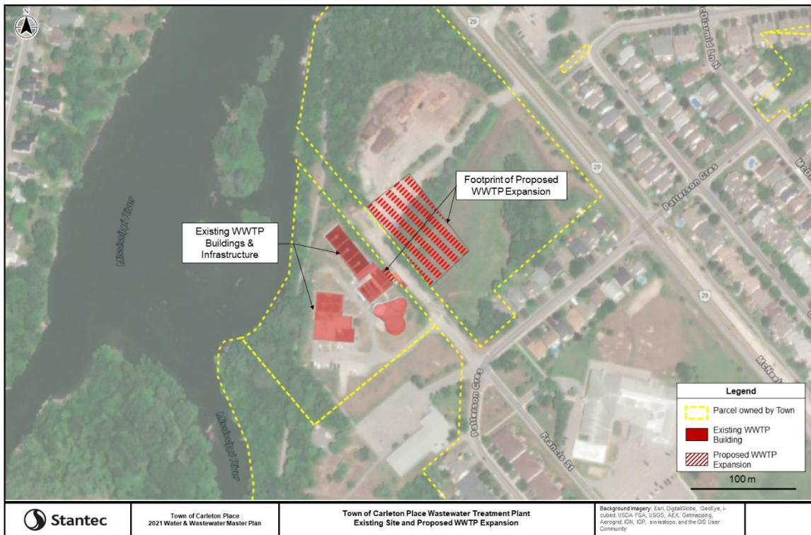
Figure 1: Potential Footprint for WWTP Expansion
