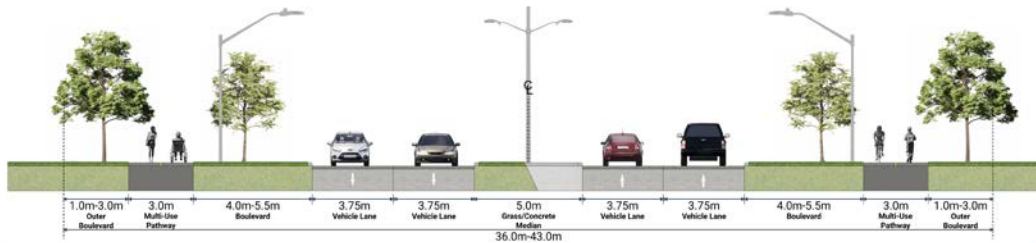
Arterial Street 26.0m Right-of-Way (Urban) New Streets and/or Future Reconstruction Option
